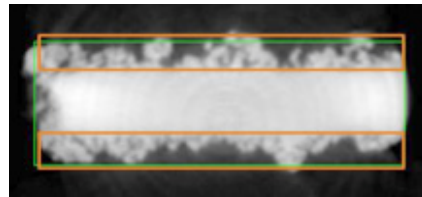
X-ray image of specimen used in the animal study. TiGrowth® coating applied to top and bottom surfaces.
